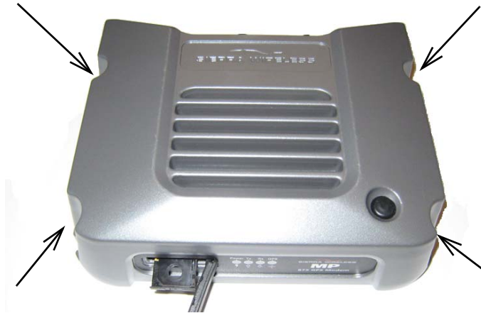
Figure 4-3: Mounting the MP modem. Arrows indicate the mounting holes. The front cover is open for illustration purposes only. Close it before mounting.
