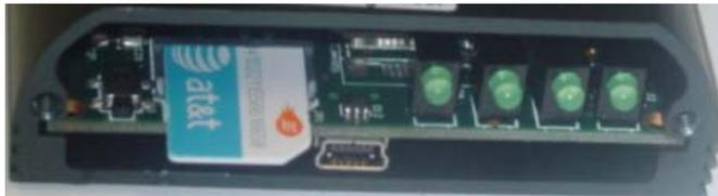
Figure 3-2: Insert SIM in to the modem
