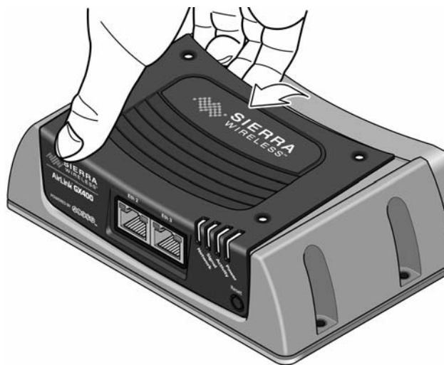
Figure 2-13: Tilting the cover (Dual Ethernet X-Card installed)
