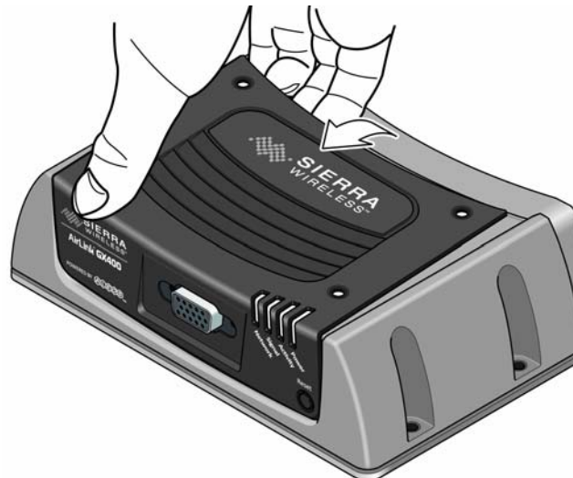
Figure 2-8: Tilting the cover (I/O X-Card installed)
