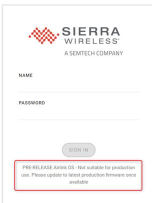
*Note: In some situations the upgrade to AirLink OS 5.0.71 from earlier versions can take up to 20 minutes. The yellow LED chase pattern followed by the green LED chase pattern indicates the upgrade is still in progress. See the [XR60 LED documentation](#). Do not remove power from the router during the upgrade.*
