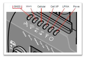
The GNSS LED is designed to indicate a detected GNSS antenna connection issue. On affected routers, the GNSS LED flashes red fast or slowly without an actual GNSS error. This is the condition this procedure is verifying.
