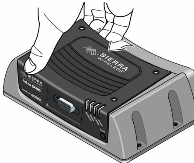
Figure 2-8: Tilting the cover (I/O X-Card installed)
