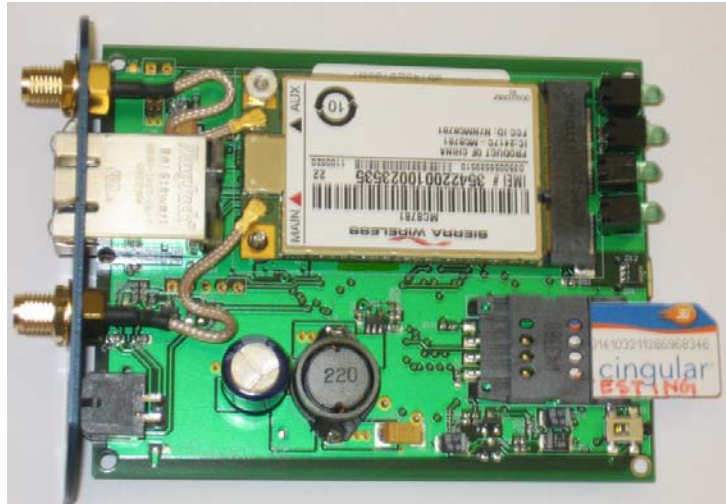
Figure 3-3: Insert SIM in to the modem
