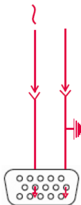
Figure 4-12: A sensor wired to Pin 7 (analog input) and Pin 10 (Ground).
