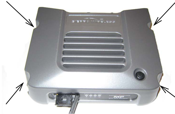
Figure 4-3: Mounting the MP modem. Arrows indicate the mounting holes. The front cover is open for illustration purposes only. Close it before mounting.
