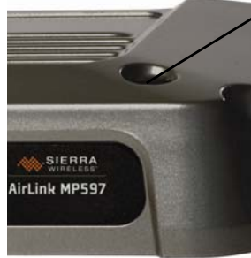
Figure 5-2: The MP modem reset button.
