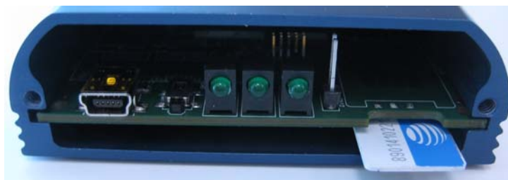
Figure 3-3: Inserting the SIM
