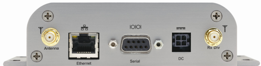
Figure 4-1: Raven X Connectors
