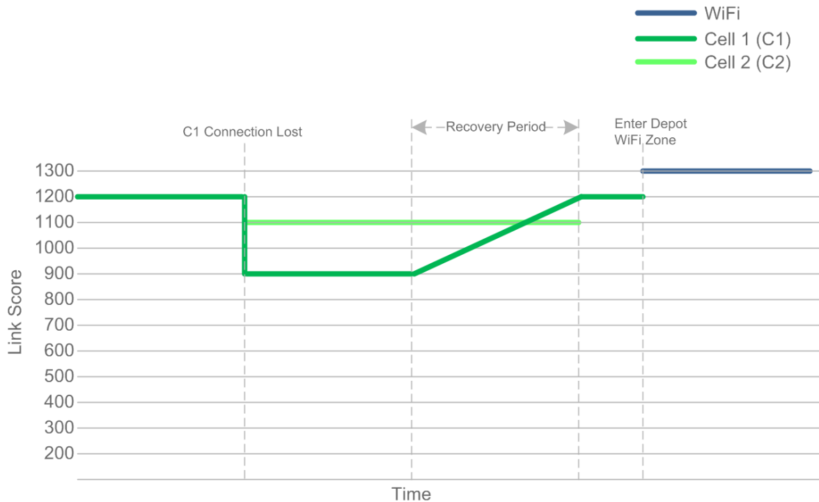
Figure 5-10: Basic example with WiFi and two Cellular links
